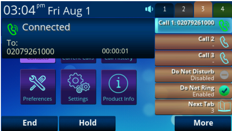
Figure 14: Tab 3 active with a call in progress on VLK 13, which is the first line key of tab 3 on the OBi1062. Note the active VLKW is highlighted and the icon shows a call is in progress.
