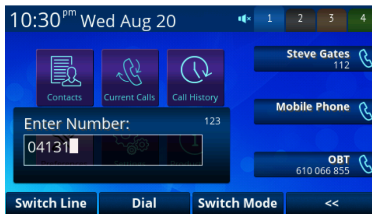
Figure 21: A phone number being entered during on-hook dialing. The digit map is not applied until the user presses the dial button.
