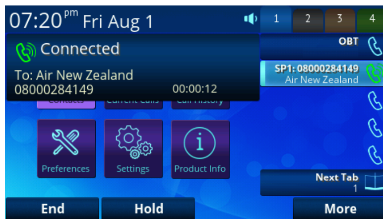
Figure 16: In this example, SP1 has no bound call keys, so when a call is made via this service an unbound call key is used. In this example, line key 1 is
